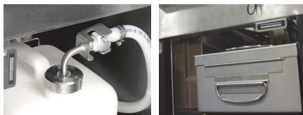
Oil replenished automatically from JIB for multi-well (left) or reservoir for 1-well (right)
